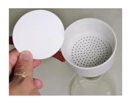
Before starting the filtration, a suitable round filter paper is placed on top of the porous plate inside the funnel.
