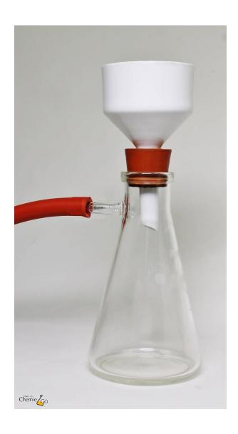
The side-arm flask is connected to a vacuum pump with a rubber tube. The rubber tube should not be fixed with a clamp.
