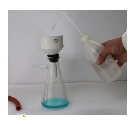
To clean the filter cake, the rubber tube is removed (keeping the pump running) and the washing solution is poured onto the filter cake.
