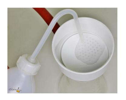
The filter paper is moistened with the solvent, in this case water.
