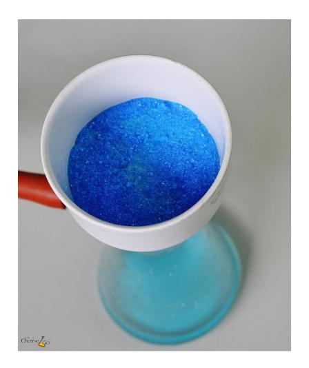
The vacuum tap is opened so that the filter paper is sucked in. Subsequently, the suspension is added. The formed filter cake additionally has a filtering effect.
