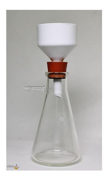
A rubber gasket (Büchner ring) is placed on the funnel which is then positioned on the vacuum flask.
