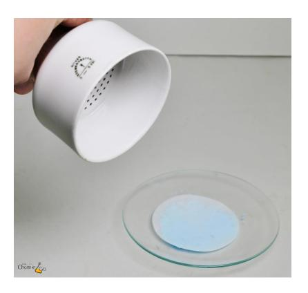
The filter cake is put on a watch glass or petri dish and the moist filter paper removed with tweezers.
